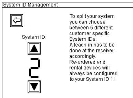
Here system ID 2 has been selected. If you change the system ID of the controller you have to teach the receivers which should respond to the commands of this controller to the new system ID afterwards (i.e. Teach-in).
