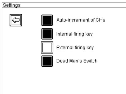
By pressing the buttons 'Auto-increment of CHs', 'Internal firing key', 'External firing key' and 'Dead Man's Switch' the corresponding function will be activated or deactivated.
