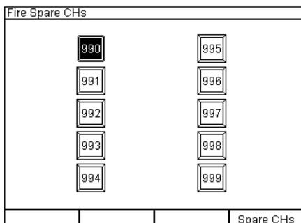
Ten channels, from 990 to 999, are intended as spare channels. Each time after switching the device on channel 990 is preselected as current spare channel. Now you may preselect another spare channel, which should be fired first. But the spare channel can still be selected also if the firing mode has been activated.
