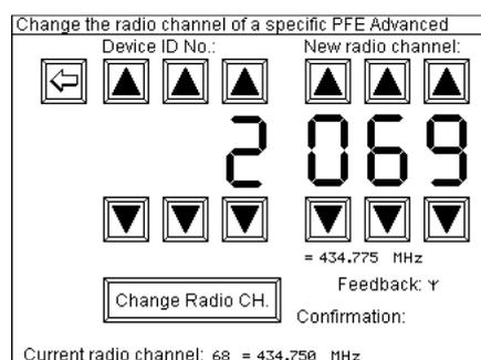
The first step is to enter the new radio channel for the receiver. This example shows that the radio channel is being changed from 68 to 69. Right beneath the radio channel the frequency in MHz is being displayed. Then enter the device ID number of the receiver that you want to address.
