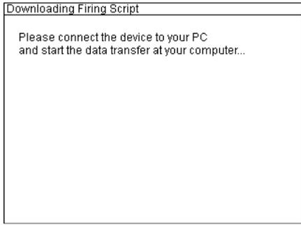
You will see this screen afterwards. Now establish the connection between the RS232/V24 port of the PFC Advanced which and the serial port of your PC by using a serial data cable. Then you can start the data transfer in the Galaxis PYROTEC Composer software. Please read also the manual of the software regarding this.
