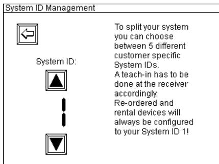
This is the default setting of the controller when being delivered to the customer. System ID 1 is selected. All re-ordered devices or rental devices will be delivered with this setting.
