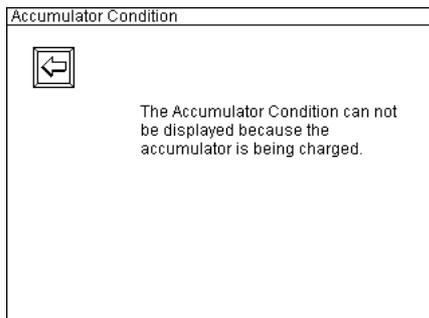
This example shows the message screen, which informs you that the battery is being charged right now. No measurements to determine the battery condition are possible during that.
