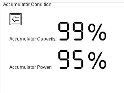
After pressing the button 'Accumulator Condition' the battery is being tested and accumulator capacity and accumulator power is being displayed.
