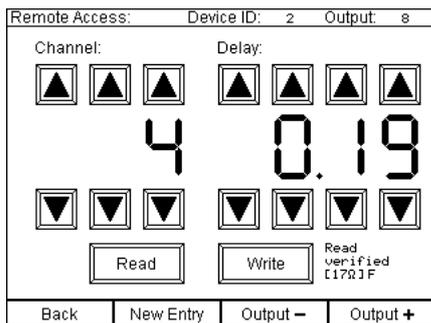
You see the information, which has been just received, being displayed and the text 'Read verified' is visible in the lower right section of the screen. As long as you can see this text you now that the information on the screen is consistent with the programming of the receiver.
