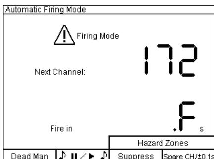
Channel 171 has been fired by the automatic fire function and channel 172 is the next cue. Apparently, no firing delay has been programmed and therefore the device waits for your manual firing by pressing the key 'Fire'.
