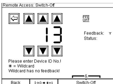
According to the symbol next to 'Feedback' you know if the device will expect to receive the feedback signal either via radio or via cable. You can determine this when selecting the device ID in the menu 'Remote Data Request' and 'Remote Programming'.
