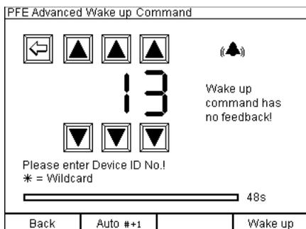
The 'Wake up' function is the opposite of the Sleep Mode. Receivers that are sleeping can be woken up by choosing the device ID of the receiver you want to wake up again. The 'Wake up' command has no feedback for technical reasons.
