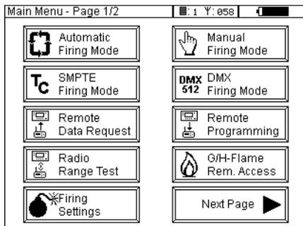
The device is in the main menu, page one is being displayed. By pressing the button 'Next Page' you will enter page two. The accumulator charging level is being displayed always in the battery symbol in the upper right corner of the screen. In this example the remaining capacity is approx. 90%.
