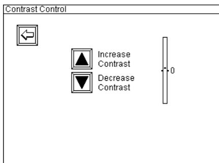
An adjustment of contrast may be required if you have difficulties in reading the information on the screen. By pressing the buttons, the contrast is increased or decreased. The selected setting is stored automatically and will be present the next time the device is operated.
