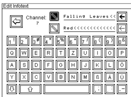
An information text of two lines (16 characters each) may be assigned to every firing channel by this function. Furthermore, you can edit information text which is already existing (e.g. information texts from a firing script which has been downloaded from the Galaxis PYROTEC COMPOSER).
