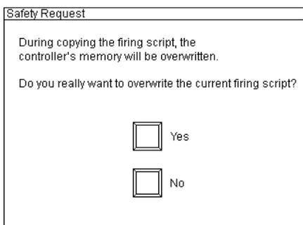
This function is required if you want to download firing scripts, which have been designed by the Galaxis PYROTEC COMPOSER, from your PC to the PFC by using the USB interface.
