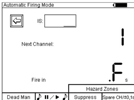
As long as the key switch 'Firing Mode' is off you cannot send a firing command. This means that you can work in this mode without any danger. In the example shown on the left the Dead Man's switch has been activated. If this function has been deactivated the text 'Dead Man' does not appear and the key is not illuminated.
