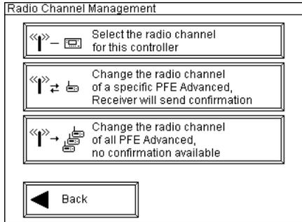
First of all, you can determine the radio channel of the controller. In addition, you can send a command to the Advanced receivers to change the radio channel.
