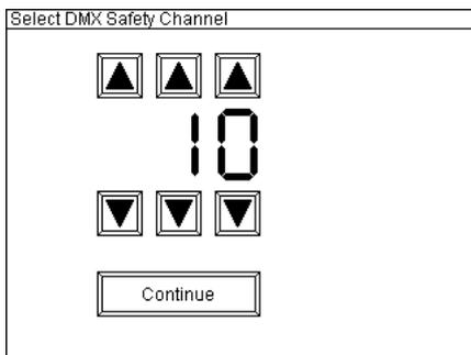
If the function 'Auto-increment of CHs' is active, the firing channel is automatically increased by one channel after ignition. If the function is switched off, the same channel will be fired again and again. The firing channels must have been programmed beforehand on the receivers or G-Flames.
