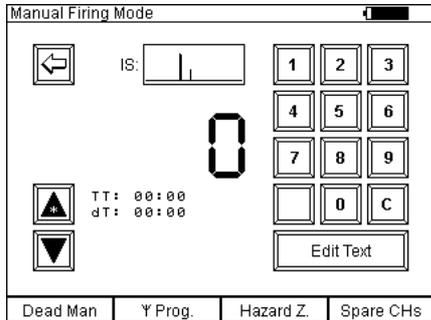
As long as the key switch firing mode is in 'Off' position no firing can be initiated. This means that you can work in this menu without any danger.
