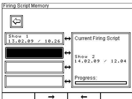
The second memory location from the top has been selected. Press the second button from the right again to copy the new script into the marked memory location.
