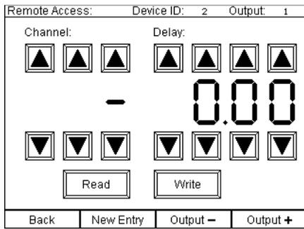
In the headline of the edit screen the device ID number of the accessed receiver and the currently selected output number is being displayed always. For a start the controller sets the output number to 1 each time when entering this mode.
