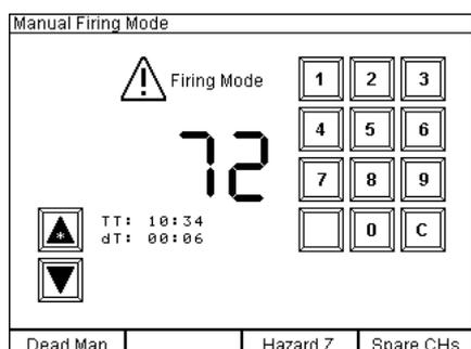
The stop watch is started after entering the manual firing mode with the first firing of any firing channel. The counting of the total time and interval time is started simultaneously.
