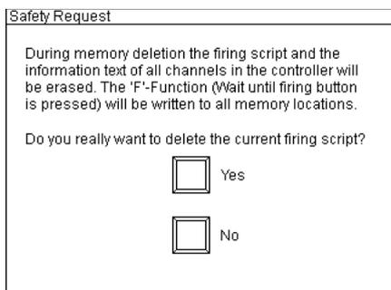
This screen is being displayed after pressing the button 'Delete Firing Script'. If you press 'Yes' all script data, including information texts, which have been entered possibly, will be deleted. All firing delays will be set to 'F' (Wait until firing button is pressed). During the process of deletion, a progress bar will be displayed.
