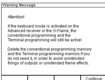
After selecting the Keyboard Mode option in the submenu of the DMX Firing Mode, the PFC asks for the first DMX channel of a group of ten DMX channels to be used. As an example, we use DMX channel 1 to 10 as control channels. After that you have to select which DMX channel should be used as safety channel. The safety channel must not be within the 10 control channels.
