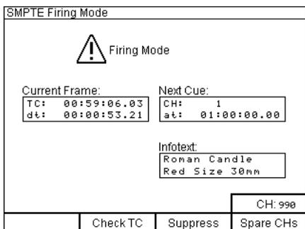
Here the firing mode has been activated. Besides the current time code you see also the time to the next cue being displayed (i.e. delta time, dt).
