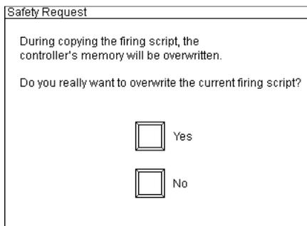
This function is required if you want to download firing scripts which have been designed by the Galaxis PYROTEC COMPOSER from your PC to the PFC by using the RS232/V24 interface.
