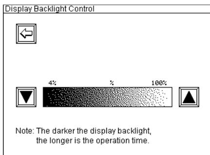
In this menu you can adjust the display backlight. A brighter display will increase the battery discharge, a darker display backlight will reduce it. The setting will be stored in the memory. When you restart the device, the last setting will be used. When switching on the device, the start screen will be shown in full brightness. After continuing to the main menu, the stored brightness value will be used.
