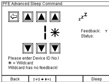
It is also possible to put more than one receiver into Sleep Mode at once. To do so, you can use a so called 'Wildcard' as a placeholder. If you want to put receivers with the device numbers 10 to 19 into Sleep Mode, you would enter the following: 0 (blank) for the hundreds, 1 for the tenths and the '\*' symbol for the wildcard. If you press 'Sleep', all receivers from 10 to 19 will be put into Sleep Mode.
