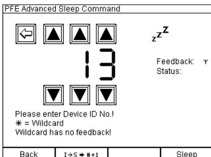
To put a receiver into Sleep Mode you have to choose the device ID of the receiver. After selecting a device ID and pressing the button for 'Sleep' the sleep command will be transmitted to the device which will send an acknowledgment. The status can be seen on the right side of the screen.
