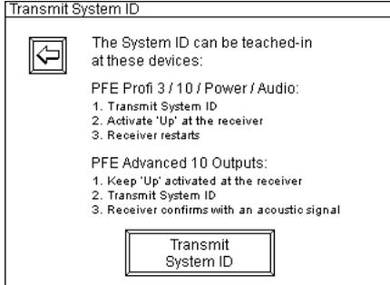
Every time you press the button 'Transmit System ID' on the touch screen the controller will transmit a command and all receivers which receive this will store this ID and they will only respond to this specific system ID in future.
