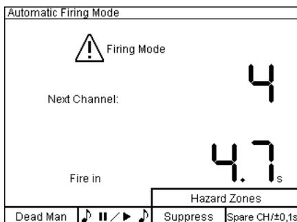
You have reached firing channel 4 in the automatic firing mode. According to the countdown timer this channel will be fired in 4.7 seconds.
