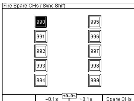
In the automatic firing mode, the spare channel button has two functions and is renamed to 'Spare CHs +/- 0,1s'.
