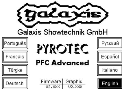
After switching the device on by turning the key switch 'operation' this start screen is being displayed. On this screen you can see, which firmware version and which graphic file has been installed. As long as you see this screen, you may choose one of the languages being displayed. After a short period of time the device enters the main menu automatically.
