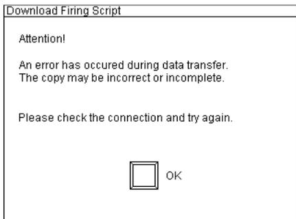
If the analysis of the check sum led to any non-conformance or the connection has been interrupted this message will be displayed. In this case you should check the connections, then press 'OK' and retry to transfer the firing script.
