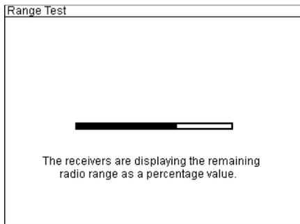
The function 'Radio Range Test' is required if you are using receivers of the 'Profi' series. These receivers do not operate bi-directionally. As a matter of course you may use this function also with receivers of the 'Advanced' series.
