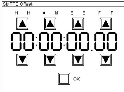
As described in the introduction of the SMPTE firing mode 00:00:00.00 should not be used as start time. Choose a frame that is far later which enables you to begin with playing back the SMPTE track including the leader without transmitting the overflow from 23:59:59:24 to 00:00:00.0.
