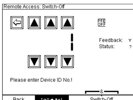
With the multifunctional key 'I->0 -> #+1' an automatic increment of the device ID can be realized. This comes in handy if a significant number of devices are in use. Then only the keys for 'Switch-Off' need to be pressed repeatedly. This function is not available in conjunction with wildcards.
