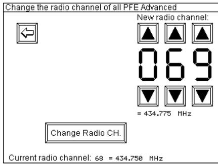
Select the new radio channel that the receiver(s) should use from now on. Right below the digits of the radio channel the related frequency in MHz is being displayed.
