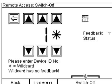
It is also possible to remotely switch off more than one receiver at once. To do so you can use a so called 'Wildcard' as placeholder. If you want to wake up receivers with the device numbers 10 to 19, you would enter the following: 0 (blank) for the hundreds, 1 for the tenths and the '\*' symbol for the wildcard. If you press 'Switch-Off', all receivers from 10 to 19 will be switched off.
