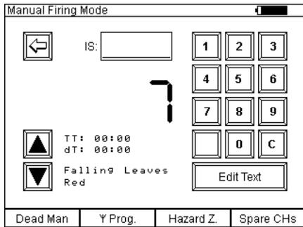
As soon as you return to manual firing mode you see the information text, which has just been entered. Information text is also being displayed if the firing mode is active. The information text is likewise valid for all various firing modes, i.e. information text, which has been entered in manual firing mode will be shown in the automatic firing mode and in the SMPTE timecode firing mode as well.
