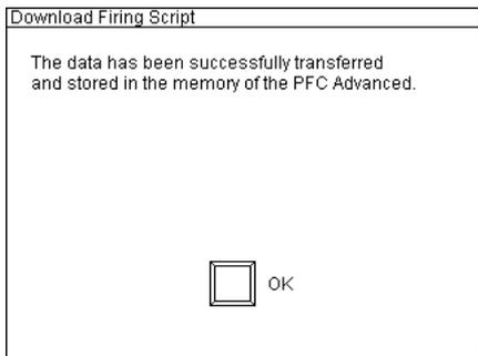
If the data has been transferred successfully you will see this screen. The correct transmission is proved by a complex check sum so that you can be sure that your firing script has been loaded by the PFC without any errors if you see this message. Press the button 'OK' to return to the submenu of the automatic firing mode.
