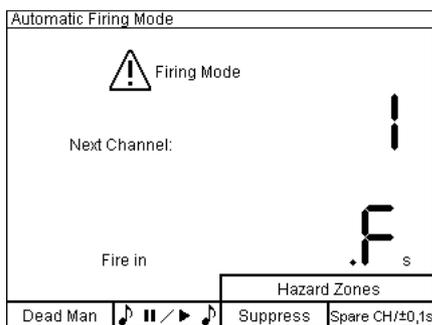
After activating the key switch 'Firing Mode' the display content changes and you see 'Attention Firing Mode' on the screen. This information in the display and the flashing firing key indicates that the device is armed.
