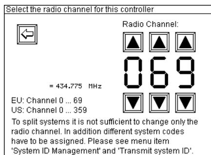
In this submenu you may select the radio channel, i.e. the frequency, which is being used for wireless data transmission.
