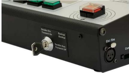
You need e.g. two PFC Advanced controllers which have been equipped with the backup function. This is an additional key switch on the right side of the front of the device.
