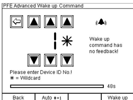
It is also possible to wake up more than one receiver at once. To do so you can use a so called 'wildcard' as placeholder. If you want to wake up receivers with the device numbers 10 to 19, you would enter the following: 0 (blank) for the hundreds, 1 for the tenths and the '\*' symbol for the wildcard. If you press 'Wake up', all receivers from 10 to 19 will wake up.
