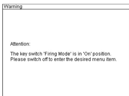
This warning message is being displayed if you enter the manual firing mode with the key switch firing mode being in 'On' position.
