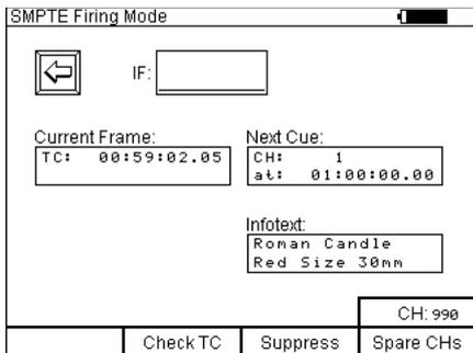
By pressing the function key 'Check TC' the current time code information is being displayed in the box 'Current Frame'. The device is refreshing this readout constantly. In the field 'TC:' you should see frames, seconds and minutes etc. counting up. Simultaneously an acoustic signal like a click sound should be audible with every frame being received.
