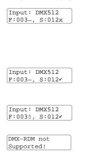
The G-Flame has been programmed to flame channel 3 and safety channel 12 ('F' = Flame channel, 'S' = Safety channel). In addition, you see the status of the safety channels and respectively of the DMX reception. 'x' means that no signal is being received or that the transmitted value of the safety channel is not within the previously configured value range (= device is not armed). The safety condition is not met in this example and no flame is being generated.
