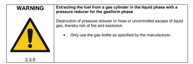
Standard pressure regulators are not suitable to be used with the liquefied phase. When the temperature is rising the pressure in the hose will increase extremely which will destroy the pressure regulator and liquefied gas is set free. Pressure regulators are offered on the market which are suitable to regulate the liquefied phase. Furthermore, a gas hose must be used that has been approved for at least the maximum bottle pressure which is 35 bar. Hydraulic hoses are suitable for this.
